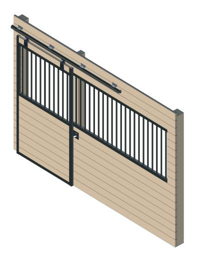
STEP 6: FINDING THE LOCATION OF DOOR KEEPERS. SHUT DOOR AND INSTALL LEFT AND BOTTOM DOOR KEEPER. OPEN STALL DOOR SO THE DOOR IS HANGING 1/2" IN STALL OPENING. THEN INSTALL RIGHT DOOR KEEPER.
