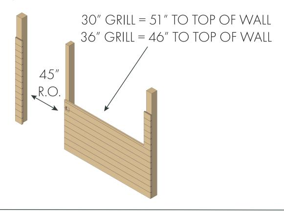
STEP 2: INSTALL GRILL. MAY NEED TO CUT GRILL TO FIT. FINISH RUNNING T&G AFTER GRILL IS IN PLACE
